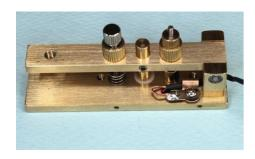
(1) Remove the dust cover, draw the cable via the thru-hole on rear side of the key. Then solder the ground core to the earth lug terminal.
