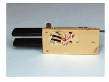
(5) Solder the red & white cable respectively with the same colored cable located in the bottom groove.
