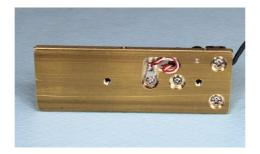
(2) Solder the center cores (red&white) on the terminal located at the groove of bottom side.
