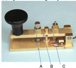
"A" for Spring Tension adjustment
